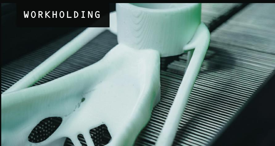
Polymorphic tools provide a precise, customised grip for complex, irregular parts, streamlining operations and eliminating the need to invest in bespoke fixtures and jigs for each product iteration.
